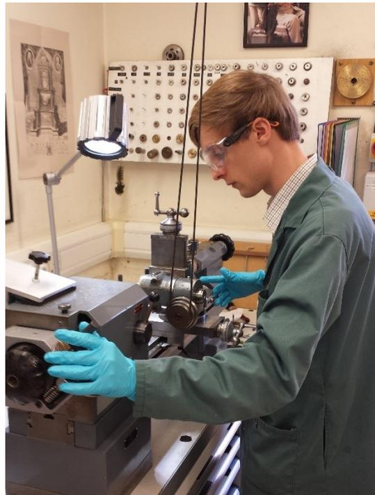
Figure 4 Using a lathe machine to make a replacement gear.
