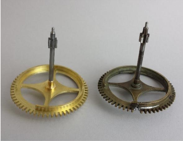
Figure 2 New wheel and pinion with its original.
