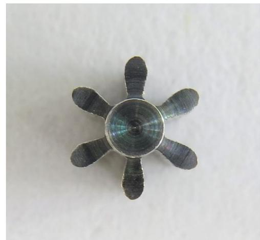
Figure 3 Close up of pinion tooth profile.
