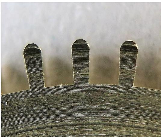
Figure 4 Close up of wheel tooth profile.
